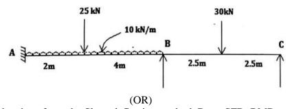
4. Analyse the given frame by Slope deflection method. Draw SFD, BMD and EC.
