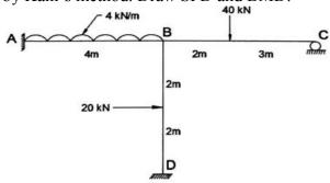
9. Determine deflection under point load. Take  $E = 200 \text{ kN/mm}^2$ ,  $I = 1 \times 10^7 \text{ mm}^4$ .
