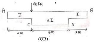
10. Determine vertical component of deflection at point C for the frame by SEM. **14M**
